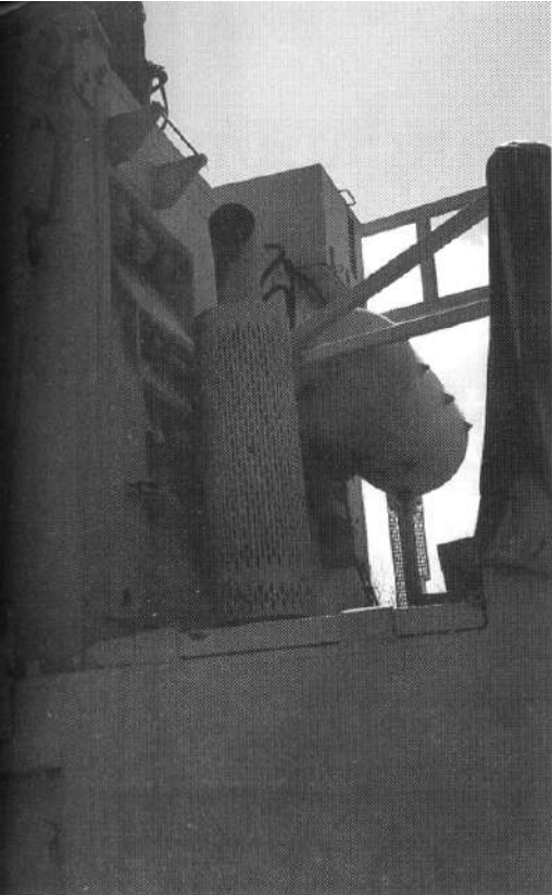
ABOVE: The exhaust and muffler in the space between the cab and the shelter box.
