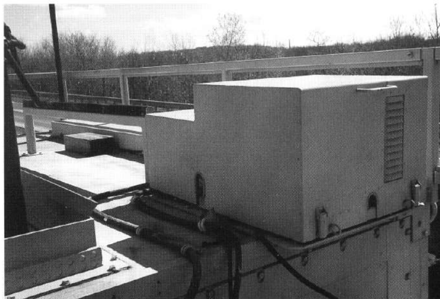
ABOVE: The exhaust and muffler in the space between the cab and the shelter box.
