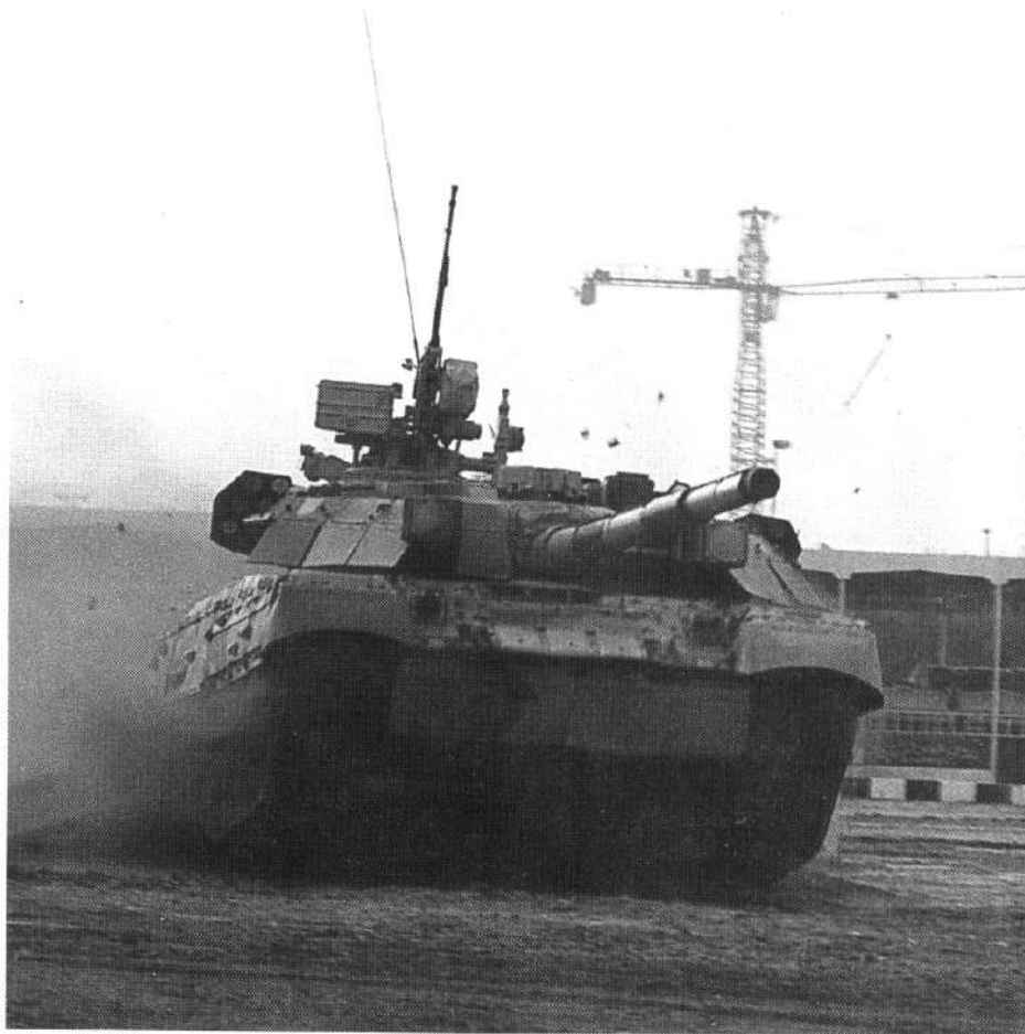
The T-84 shown here is basically identical to the T-80UD. The obvious external difference is the welded hull of the T-84.
