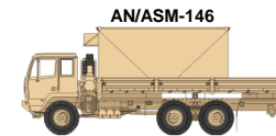
ELECTRONICS SHOP SHELTER MOUNTED AVIONICS: AN/ASM-146 (SHOWN MTD ON M1085 MTV) (H01907)
